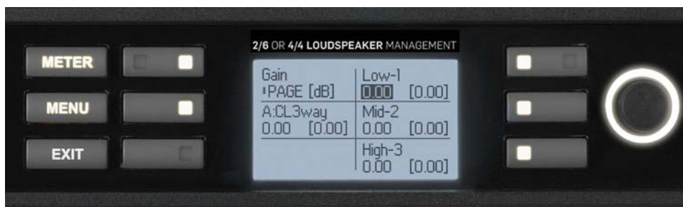
Figure 6-10: Single Module Gain Edit Screen
