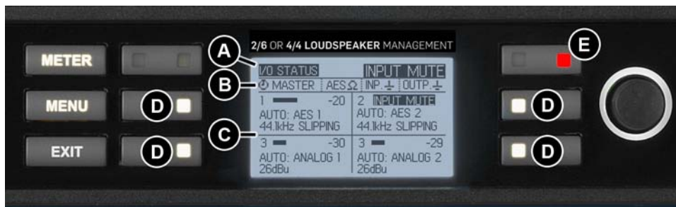
Figure 6-6: Meter Mode > I/O Status View
