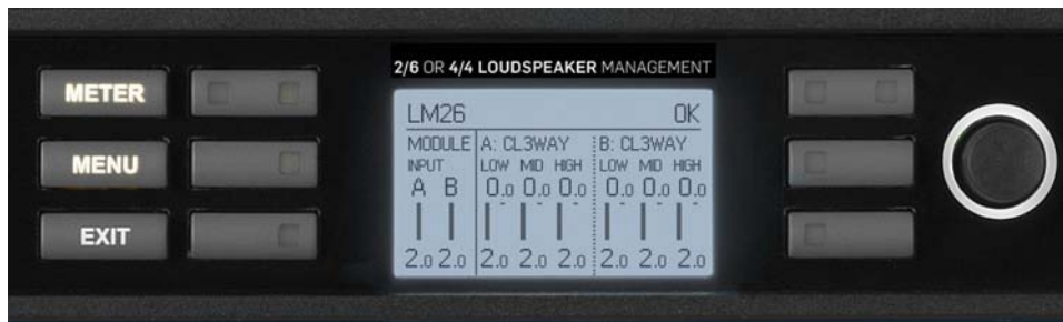
Figure 6-5: Meter Mode > Home View
