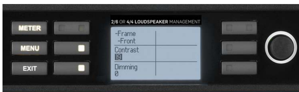
Figure 6-21: Front Panel Display Controls Menu
