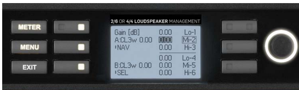
Figure 6-11: Module A+B Combined Gain Summary Edit Screen
