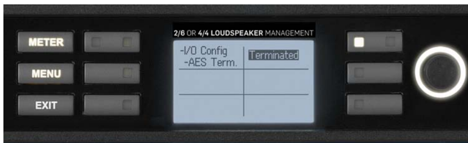
Figure 6-14: AES Termination Edit Screen
